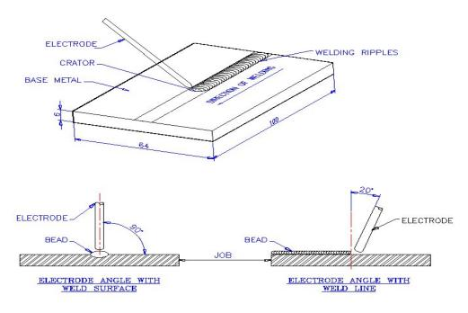
ELECTRODE POSITION WHEN MAKING ON FLAT BEAD
