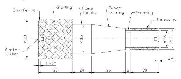
Swiveling angle = Half of the taper angle =  $4^{\circ}$ , All Dimensions are in mm, Tolerance =  $\pm 0.5$ mm
